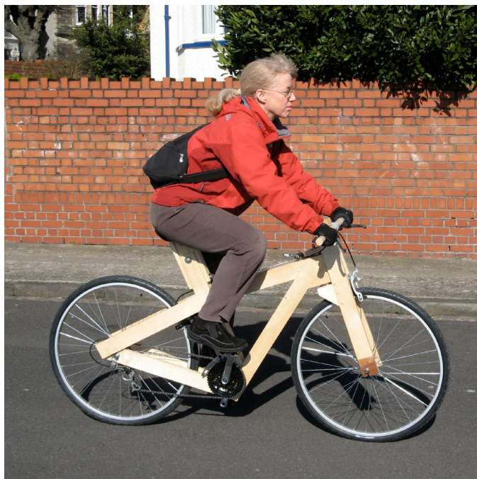
Ironwood bicycle 6, unpainted to show its construction
