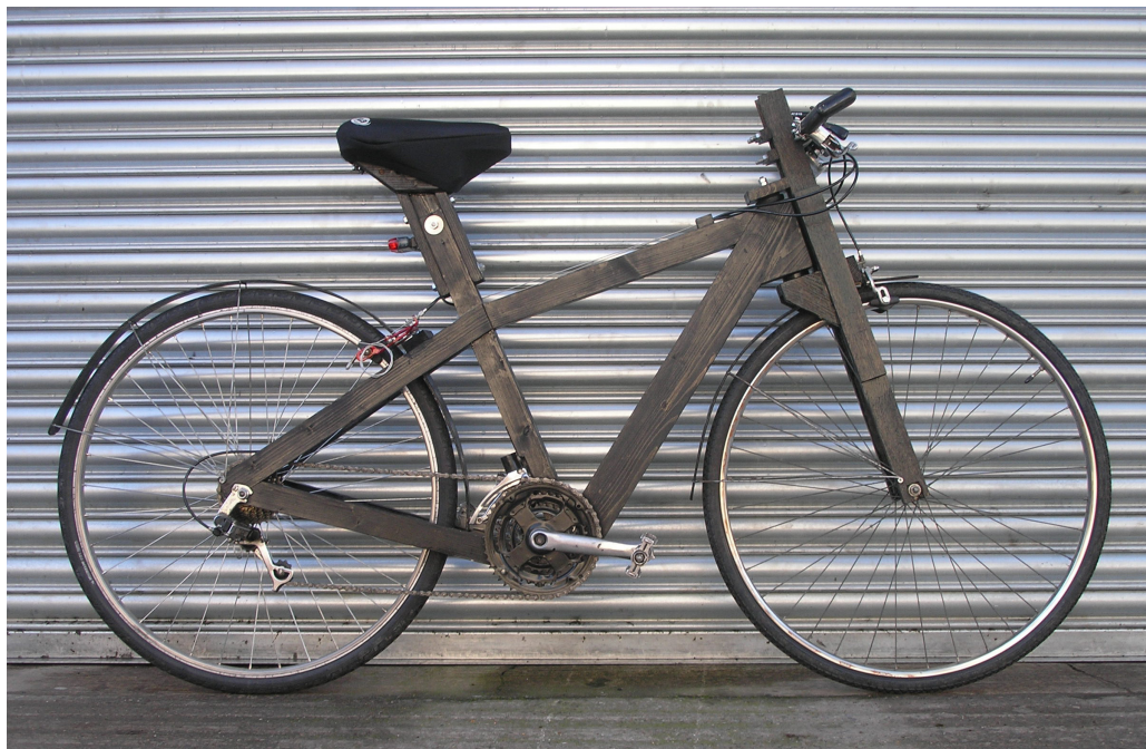
Ironwood bicycle 9 constructed with a wooden frame, fork, seat, handle bars and mudguards
